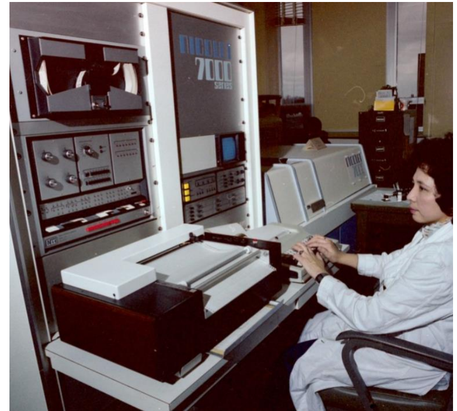
Nicolet 7000 Series FTIR Spectrometer, 1984
